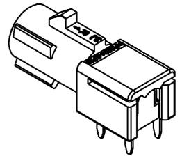
THE CONNECTOR MUST BE HOLD IN PLACE DURING THE SOLDERING OPERATION
